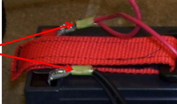
5. Disconnect the two wires from the back of the old power receptacle. Discard both the black wire and the red wire with the fuse holder and diode.
