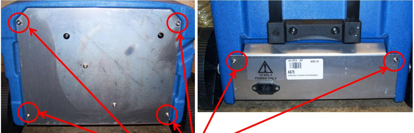
REMOVE SIX SCREWS to remove Base Plate from Sprayer Body
